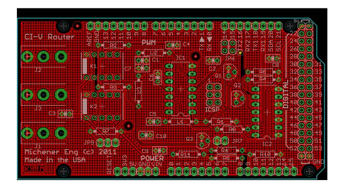
The CI-V Router board is a "shield" that plugs into an Arduino Mega 2560 board that provides the following features:
