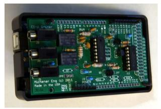
CI-V Arduino Mega shield board, built test and ready to plug in.
